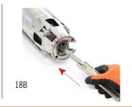
Use DEPTH CALIPER to check shaft clearance
