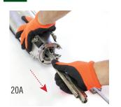
Use DEPTH CALIPER to check shaft clearance
