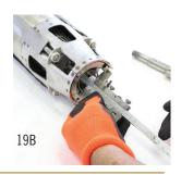
**Pull out SHAFT using DEPTH TOOL**
