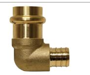
A.Y. McDonald Mfg. Co. copper press fittings are for use in plumbing or mechanical applications. Sizes range from 1/2" - 1" and the fittings are designed to join ASTM B88 (Types K, L, M) hard-drawn copper tube and soft copper tube on the press end and PEX Tubing in accordance with ASTM F876 & F877 on the PEX end.
