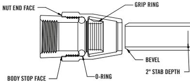
The A.Y. McDonald Series compression system is a simple convenient method of connection for tube size service materials (See table below for approved tubing specs.)
