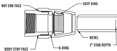
The A.Y. McDonald Series compression system is a simple convenient method of connection for tube size service materials (See table below for approved tubing specs.)
