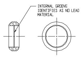
NDTE: MUST BE USED WITH COPPER TUBE OR COPPER GASKETS TO ENSURE PROPER SEAL
