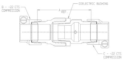
NOTE: ACTUAL LENGTHS WILL VARY DUE TO ASSEMBLY OF INSULATOR.
