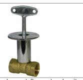
A.Y. McDonald Mfg. Co. straight and angle log lighter valves are constructed of heavy-duty forged brass. They have a teflon seat and a viton rubber synthetic fiber stem seal. The extremely high B.T.U. capacity makes them a good choice for either natural or artificial fireplaces. Valves are designed for use with natural, manufactured or LP gas only.
