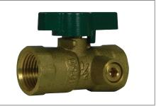
A.Y. M<sup>c</sup>Donald Mfg. Co. Gas Ball Valves equipped with a 1/8" FNPT Pilot Tap are constructed of heavy duty forged brass and designed for residential, commercial, and industrial use in low pressure gas applications. A manometer can be attached to the side tap allowing line pressure to be tested at the valve eliminated the need for a test tee and the labor to install it. Valves listed are suitable for use with natural, manufactured, mixed and LP gases and with LP gas - air mixtures.
