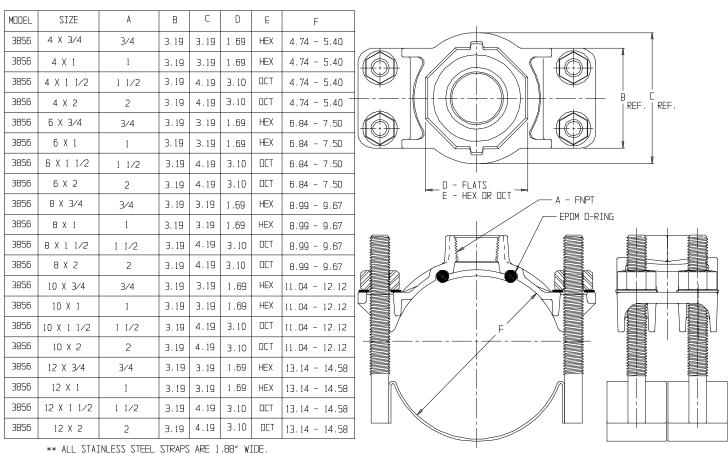
\*\* ALL STAINLESS STEEL STRAPS ARE 1.88" WIDE. TWO STRAPS (WITH 2 STUDS WELDED DN) PER ASSEMBLY
