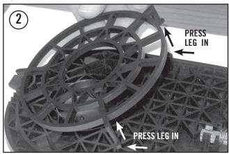
2) To remove the carriage from under side of yokebox lid for ERT attachment, gently apply pressure inward to the two locking legs and pull the carriage assembly slightly upward as pressure is applied.
