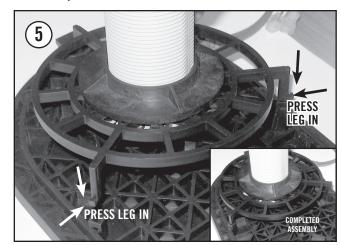
5) With slight inward pressure on each leg, push the carriage assembly down and into the locking position.
