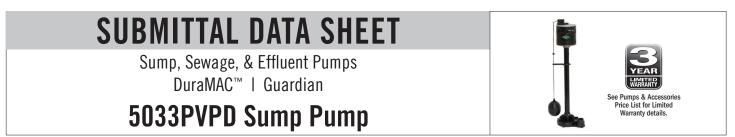
The 5033PVPD is designed for use in sump basins 12" or larger. It has a tough thermoplastic base and will handle liquids up to 120°F.
