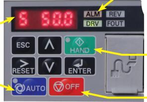
Press to turn HAND mode on. Use only for Priming and troubleshooting. Pump will run at a fixed speed.
