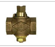
A.Y. McDonald Mfg. Co. low pressure natural or propane gas valve for use indoors on house piping system, between the meter outlet and the inlet connection of the gas appliance. At ambient temperatures of 32 to 125 degrees Fahrenheit.
