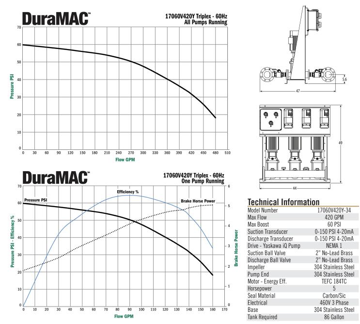
NO-LEAD: The weighted average of the wetted surface of this no-lead product contacted by consumable water contains less than one quarter of one percent (0.25%) lead.
