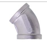
A.Y. M<sup>c</sup>Donald Mfg. Co. Pipe Fittings are constructed from 304 stainless-steel and are rated for commerical, industrial and residential applications up to 150 PSI. Threads conform to MSS-SP114 standards and specifications.
