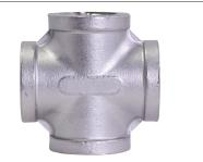
A.Y. M<sup>c</sup>Donald Mfg. Co. Pipe Fittings are constructed from 304 stainless-steel and are rated for commerical, industrial and residential applications up to 150 PSI. Threads conform to MSS-SP114 standards and specifications.
