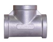
A.Y. M<sup>c</sup>Donald Mfg. Co. Pipe Fittings are constructed from 304 stainless-steel and are rated for commerical, industrial and residential applications up to 150 PSI. Threads conform to MSS-SP114 standards and specifications.
