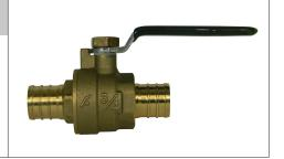
A.Y. McDonald Mfg. Co. No-Lead Ball Valves are constructed from heavy duty no-lead forged brass and can be used with potable water in commercial, industrial, and residential applications. This is a standard port valve with excellent flow characteristics.
