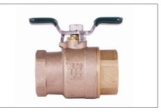
A.Y. McDonald Mfg. Co. No-Lead Full Port Bronze Body Ball Valves are constructed from heavy duty no-lead brass and can be used with a full range of liquids and gases in commercial, industrial, and residential applications. Full port valves allow for maximum flow with minimum pressure drop.
