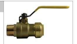
A.Y. McDonald Mfg. Co. No-Lead Push-Fit Valves are designed for use on copper tubing, Pex tubing, and CPVC pipe. Push-Fit end connections eliminate the need for soldering, crimping, or solvent welding and are designed for above ground, indoor water purposes. These heavy duty valves can be used with potable water in commercial, industrial, and residential applications.
