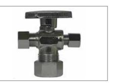
A.Y. McDonald Mfg. Co. dual outlet supply stops allow two separate supply lines to be attached to a single valve. Ideal for adding dishwashers, ice makers and more to an existing water supply. Designed to stop the flow of water running to the plumbing fixture, allowing for maintenance and repair without shutting off the water to the entire house.
