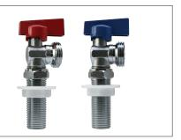
A.Y. McDonald Mfg. Co. No-Lead Quarter Turn Supply Stops are fully certified to all applicable standards. The Ball Valve design allows for ease of operation and positive shut-off and is ideal for residential and commercial applications. Each valve is constructed of heavy duty chrome plated brass.
